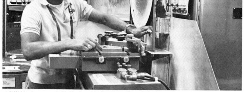
24-CARAT cuts are assured with this diamond band saw in Ceramics Lab. One of two such recently-acquired instruments, the saw can make repeated cuts accurate to within two tenthousandths of an inch (.0002"). Ceramics, quartz glass, carbon, or any other extremely hard material can be cut with ease by the 118-inch long diamond-coated band. A unique feature of
